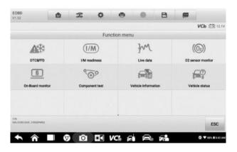
Figure 6-9 Sample OBDII Diagnostic Menu
